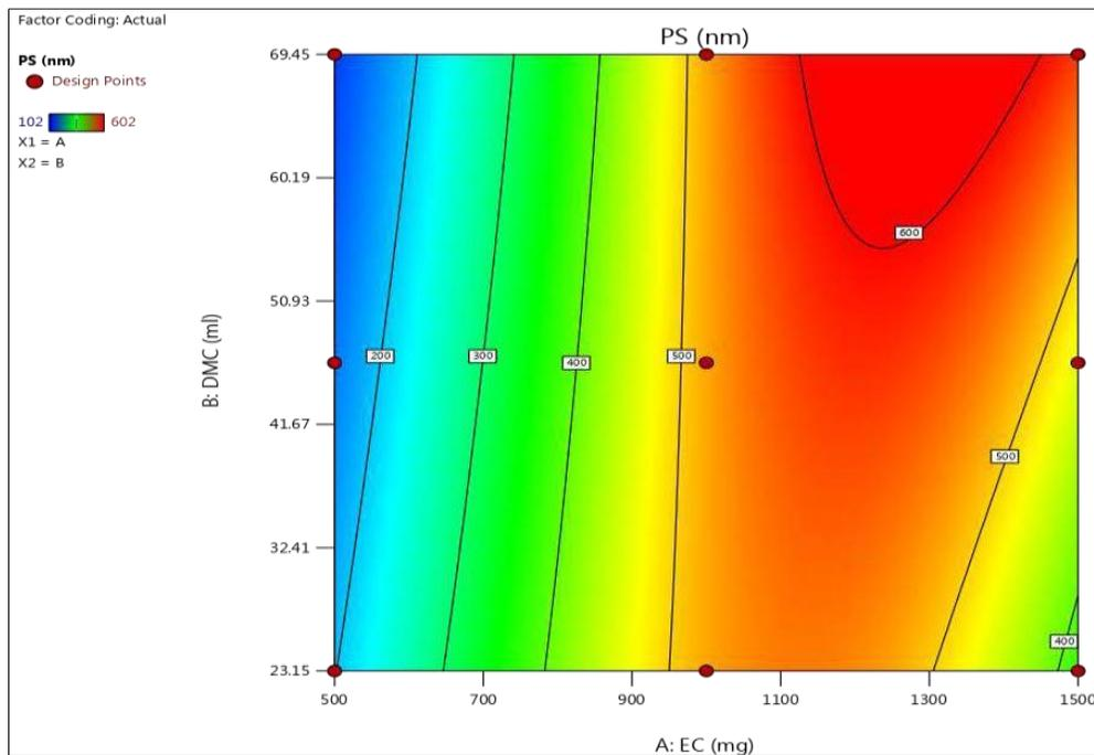
Fig 8: Counter plot showing the effect of EC and DMC ratios on the PS from formulation
