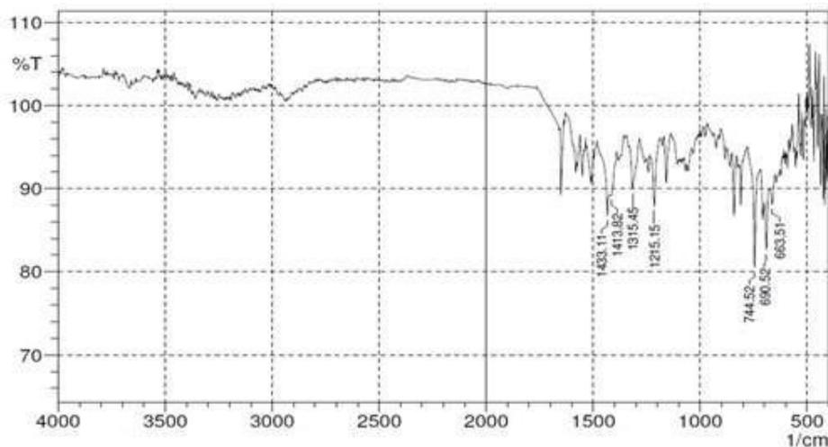
Fig 22: FTIR spectrum of freeze dried ATRC-NSGs 40°C ± 2°C and RH 75% ± 5 % after 6 months
