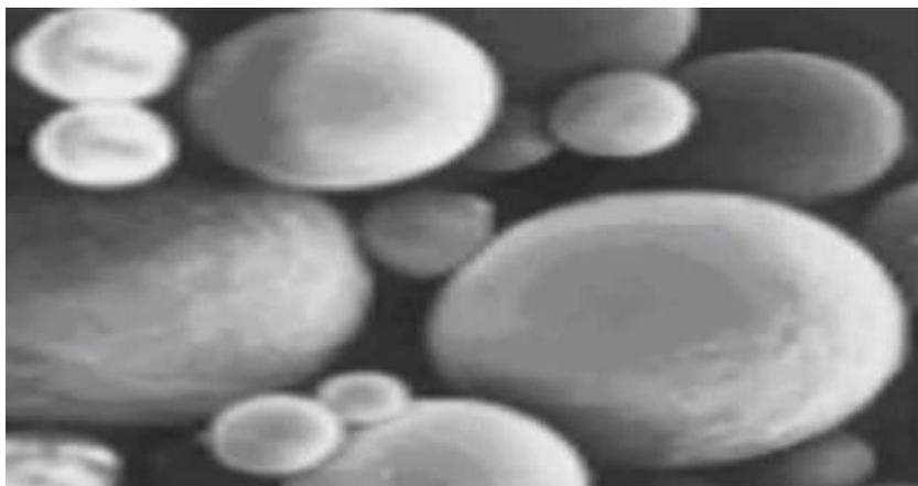
**Fig 18 : Micrographs of ATRC-NSGs by transmission electron microscope for Optimized Formulation F6 (110 nm)**
