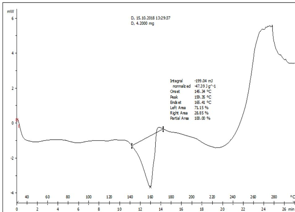
**Fig 4: DSC thermogram of Atorvastatin calcium**
