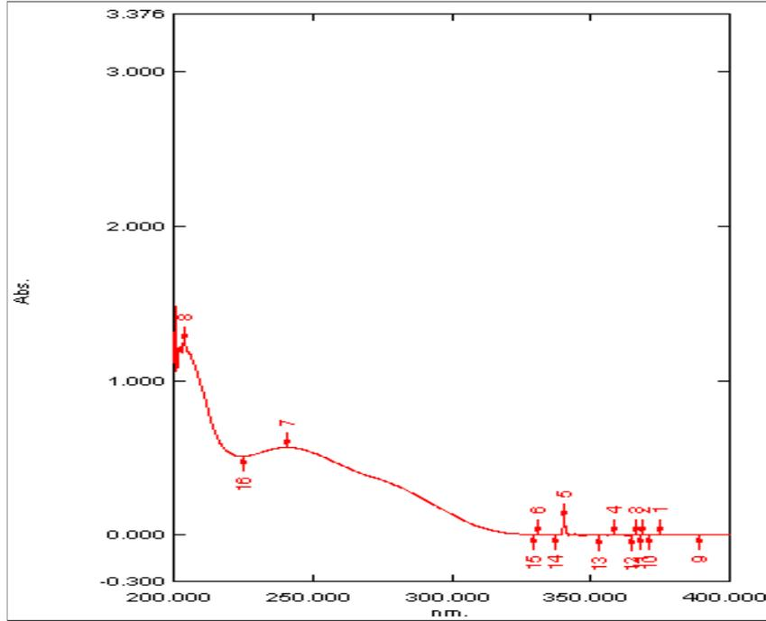
**Fig 5: UV-absorption spectrum of Atorvastatin calcium**
