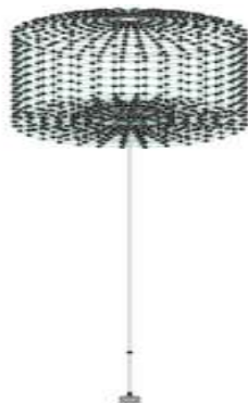
Fig. 5 Node view of Precast OHT model
