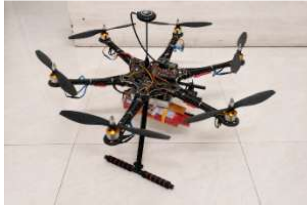
Fig. 4. Top view of the developed hexacopter platform showing six-rotor configuration, embedded flight controller, GPS module, and onboard processing unit.
