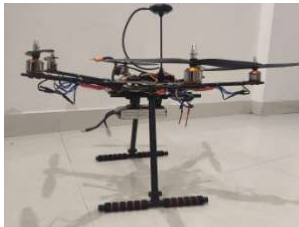
Fig. 5. Side view of the hexacopter illustrating landing gear structure, battery placement, propulsion system, and structural frame assembly
