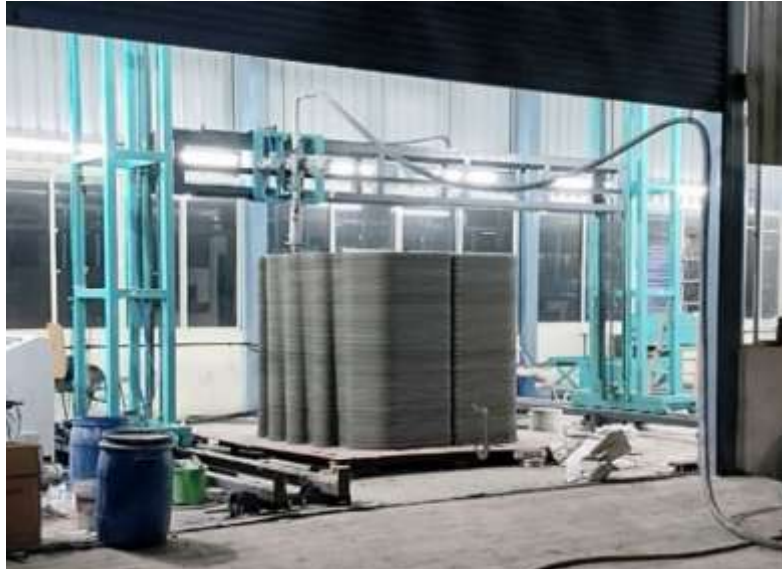
Fig. 1: Concrete 3D Printer at PCCoE, Pune
