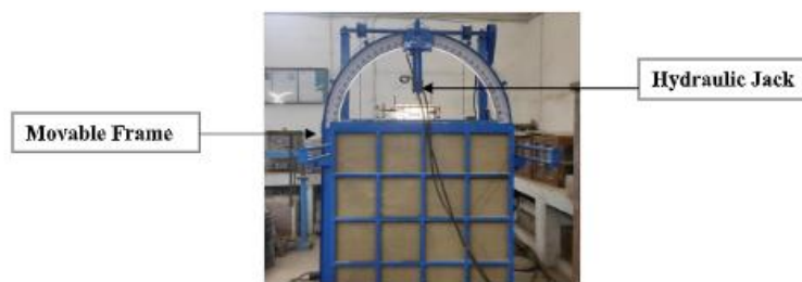
Fig 3.1: Model Foundation Tank
