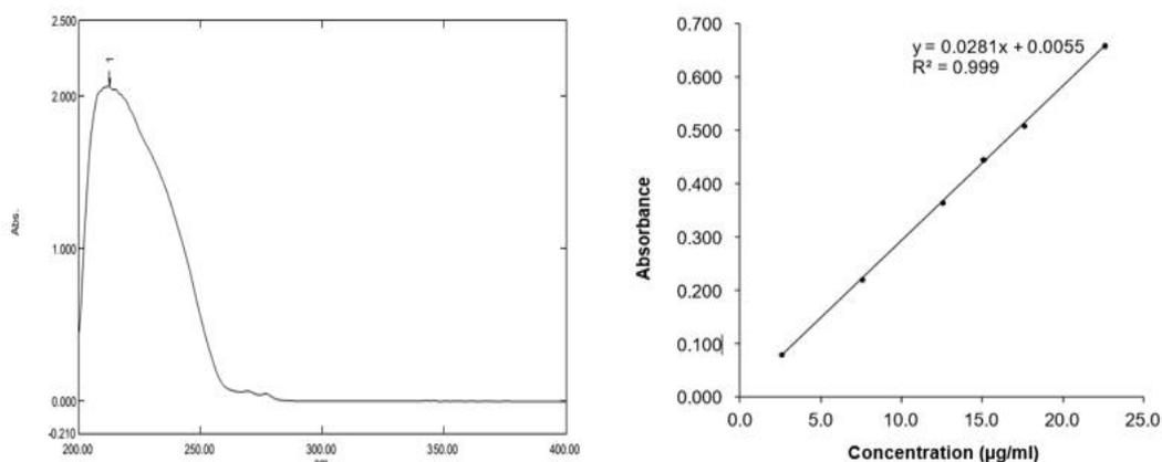
Figure 2 : UV Absorbance spectra and calibration curve of Clopidogrel in methanol
