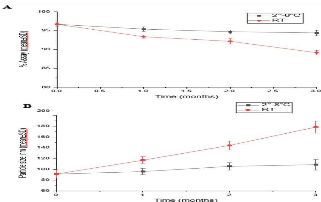
**Figure 10:** Stability of formulation (n=3); Assay (A) and particle size (B)
