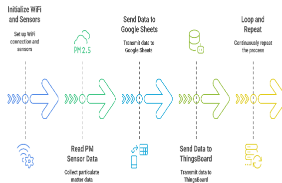
Fig.2: Air Quality Data Transmission Sequence
