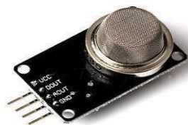
Fig.5 Air checking purity sensor (MQ135)
