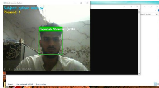
Fig-7: Live attendance session — Divyansh Sharma recognized with green bounding box, Subject: Python Lab, Present count: 1
