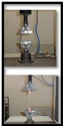
Figure-5: A) Inostron machine; B) Assembly with holding samples
