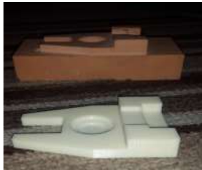
Figure 7: Machined and 3D printed model
