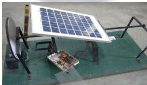
Fig. 3: Proposed assembly for the solar tracking system
