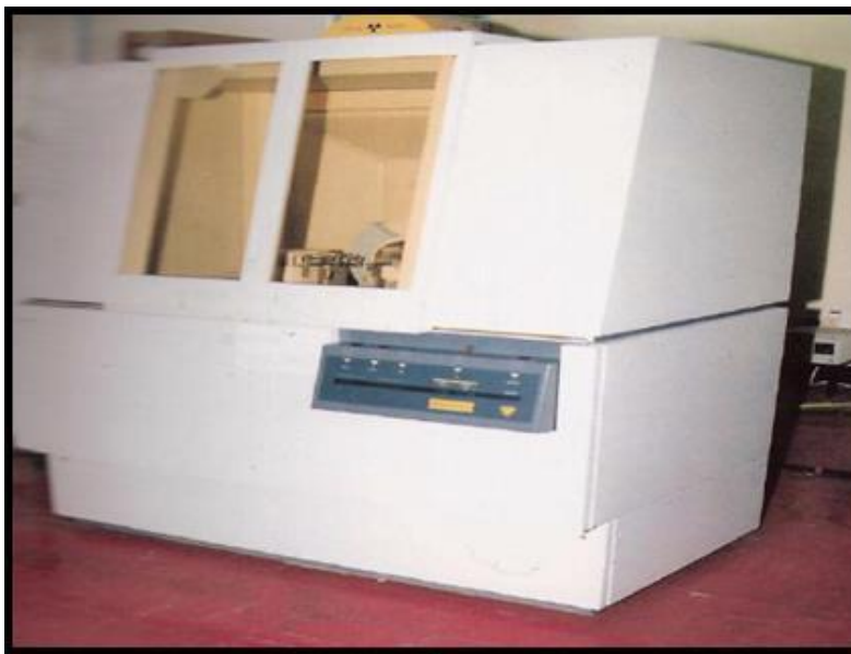
Fig.3 Philips X-pert multipurpose x-ray diffractometer
