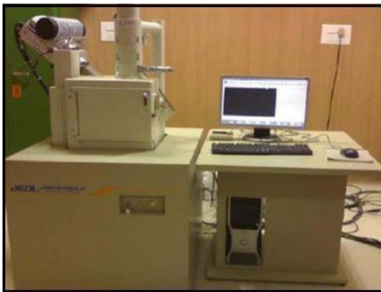
Fig. 2 Scanning Electron Microscopy (JEOL JSM-6480LV)
