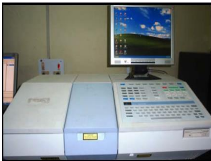
Fig.4 Perkin-Elmer Spectrum RXI, (FTIR) Spectrometer
