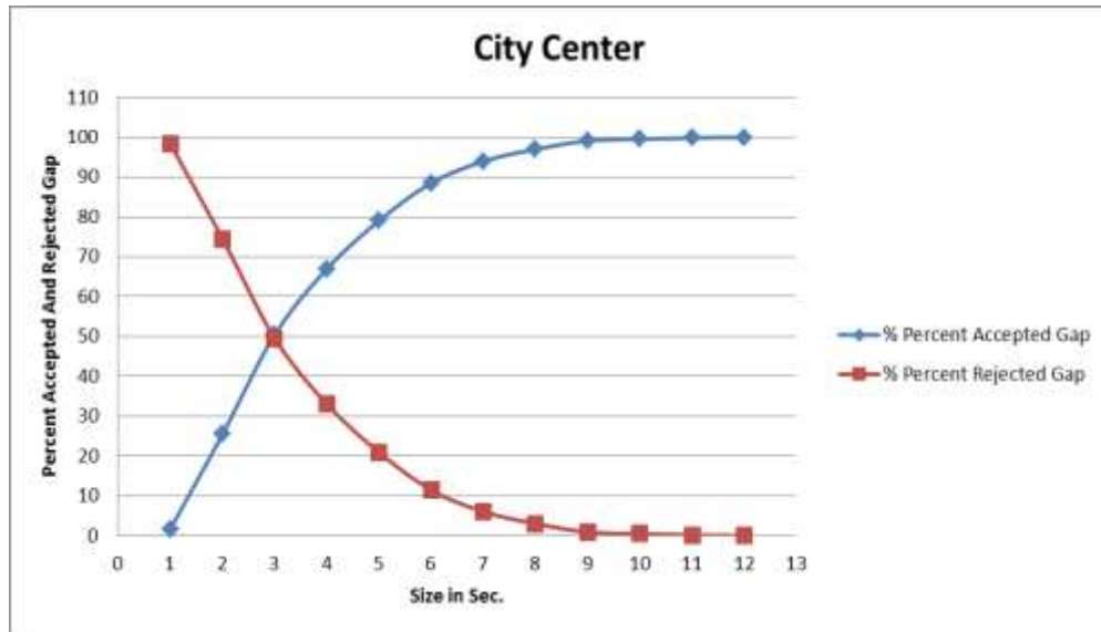
Figure (7): Accumulated Accepted, and/ or Rejected Gap on Midblock Crosswalks Located in Dohuk City CBD Area
