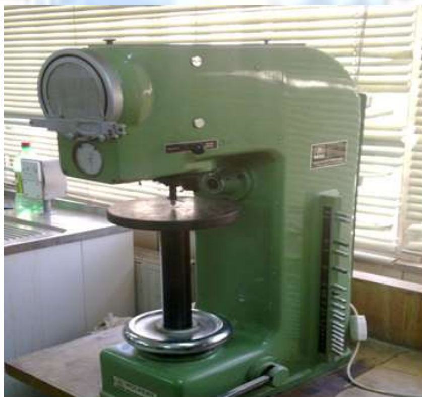
Fig (3): ( Amsler, KARL-KOLB/Germany) machine for measuring the indentation hardness
