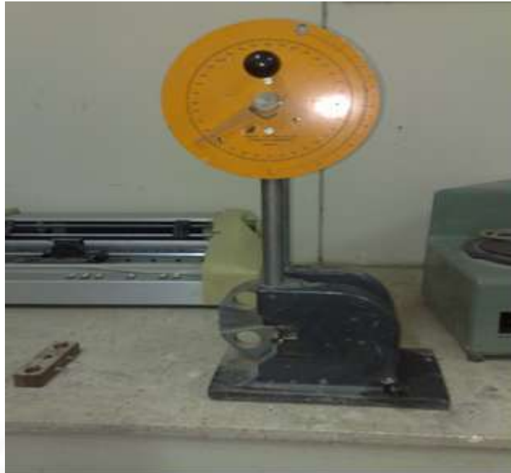
Fig (4): Charpy's pendulum impact testing machine (ZEIZZ-West Germany)
