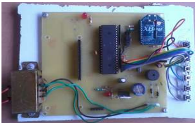
Figure IV.ii circuit of receiver module
