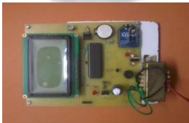
Figure IV.i : circuit of transmitter module
