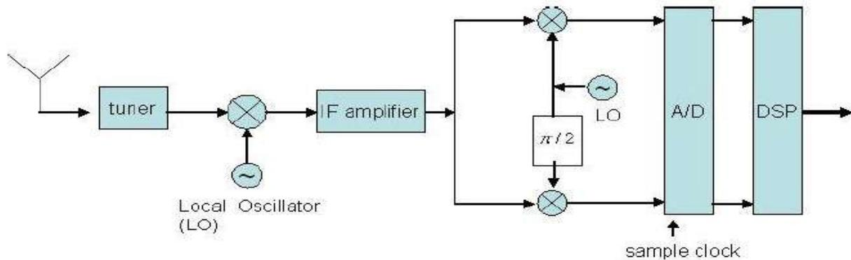
Figure 5.1 OFDM Receiver Front End
