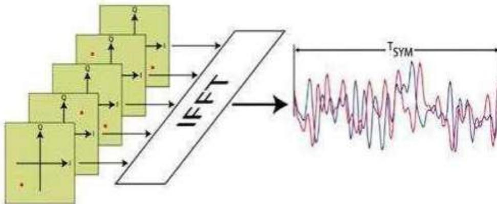
Figure 2: Transmitter implementation using IFFT
