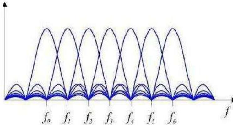
Figure 1: Bandwidth utilization of OFDM.
