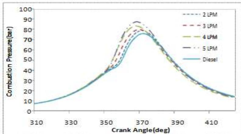
Fig. Variation of Cylinder Pressure with Crank Angle
