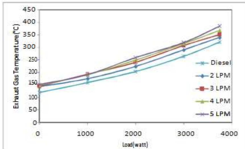
Fig .Variation of Exhaust Gas Temperature with Load
