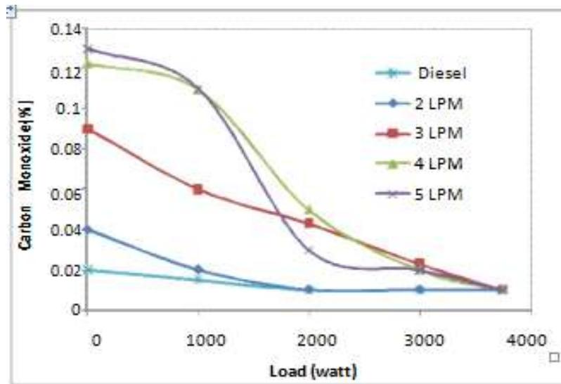
Fig . Variation of Carbon Monoxide with Load
