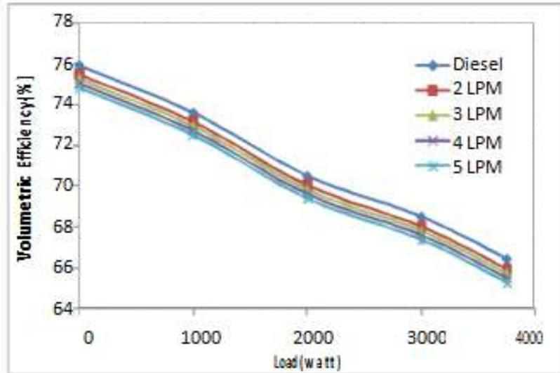
Fig .Variation of volumetric efficiency with Load
