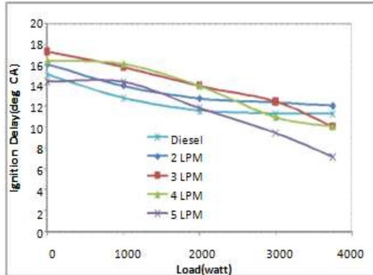
Fig. Variation of Ignition Delay with Load
