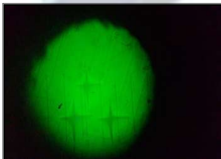
Figure (3): Three Indentations Made on Each Surface of the Sealant
