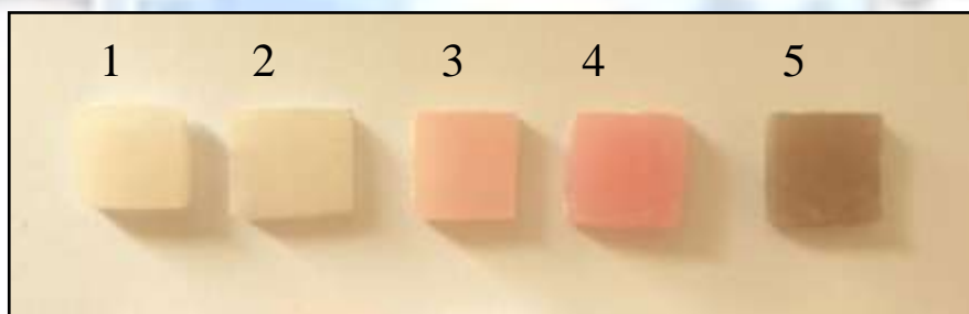
Figure (3.7): Samples of translucent heat cured acrylic with 10% wt/wt Vertex TM synthetic additives. (1): with synthetic stain No.210, (2): with synthetic stain No.220, (3): with synthetic stain No.230, (4): with synthetic stain No.240, (5): with synthetic stain No.250.
