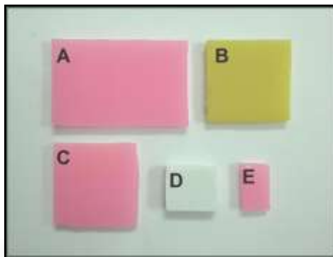
Figure (3.5): The Models of Biostar Used in the Preparation of the Samples. A: Color property measurement test sample. B: Residual monomer test sample. C: Indentation hardness and volumetric change test sample. D: Water sorption and solubility test sample. E: FTIR test sample.
