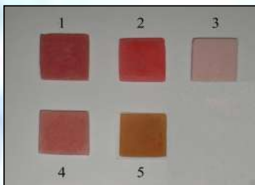
Figure (3.8): Samples of pink heat cured acrylic with natural pigments in different concentrations. (1): Amaranth 0.1%, (2): Raspberry 0.01%, (3): TiO 2 1%, (4): Vanilla 10%, (5): Curcumin 1% wt/wt.
