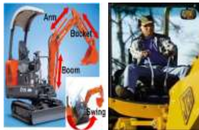
Fig 3.1 Excavator degrees of freedom
