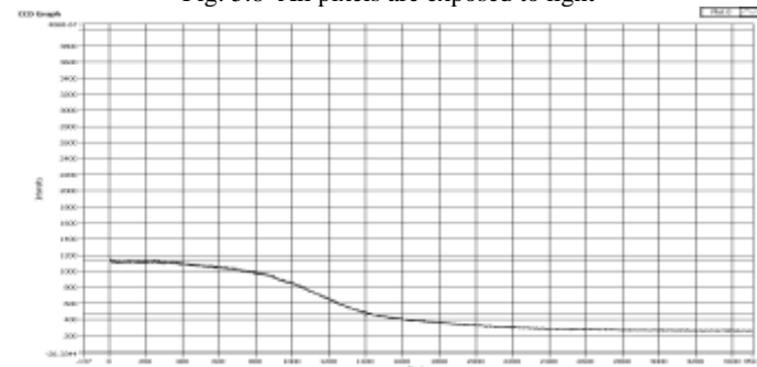
Fig: 5.9 Graph of light intensity w.r.t pixels when CCD is moved towards the right extreme end of the field of view
