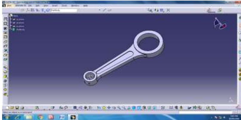
Figure 3 CAD model of Connecting Rod in CATIA V5
