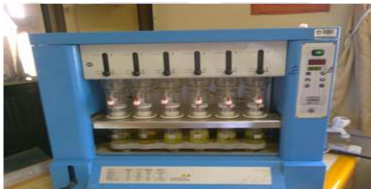
Fig. (1): Solvent Extractor apparatus
