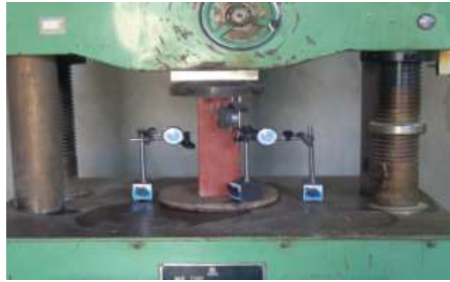
Figure 1: Test setup of stub columns
