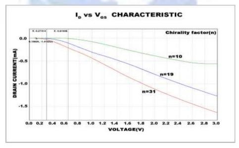
The above graph shows that as the chirality factor increases in a CNTFET
