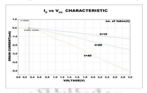
The above graph shows that as the number of tubes increases in a CNTFET:
