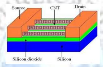
The threshold voltage of CNT channel is approximately equal to the half of the band-gap and varies inversely with diameter.
