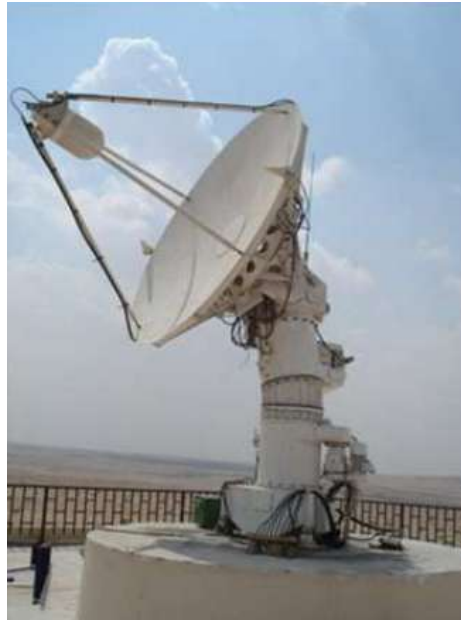
Figure 1. Az-El- Tilt pedestal
