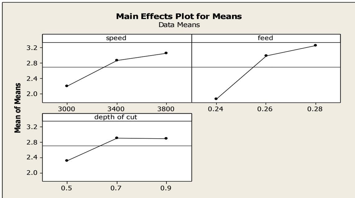
**Fig.5- Main effects Plots for Means of Ra**
