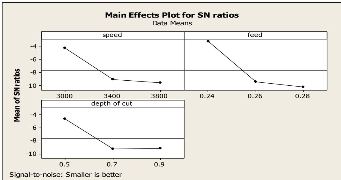
**Fig.6- Main effects Plots for S/N ratio of Ra**
