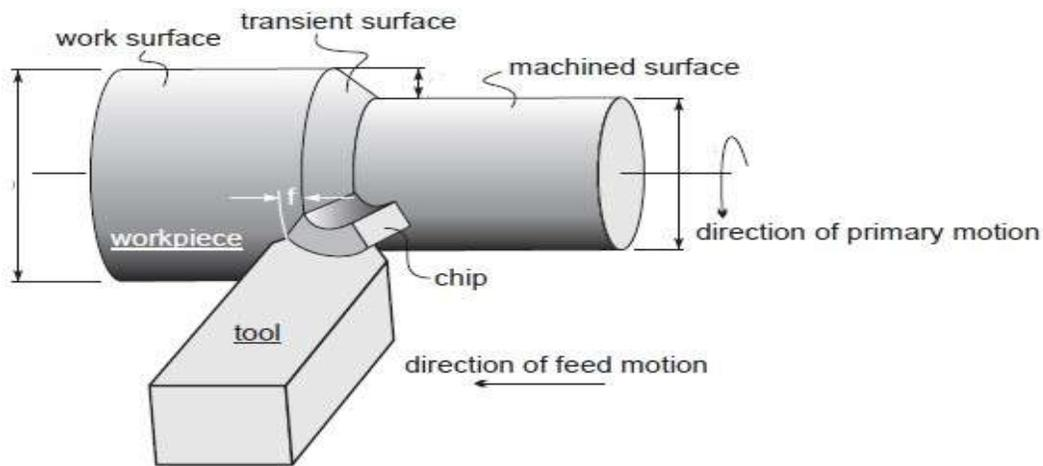
**Fig.1- Symmetric view of basic turning operation [IITB]**
