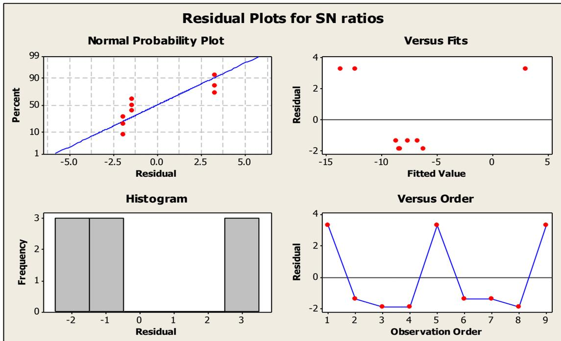
Fig. 8- Residual Plots for S/N ratio of Ra
