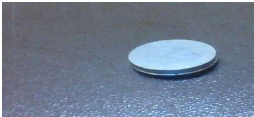
**Fig.2-Work-piece specimen material case hardening steel 16MnCr5**
