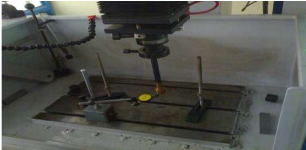
Fig III. To check level of the lower surface of the copper electrode
