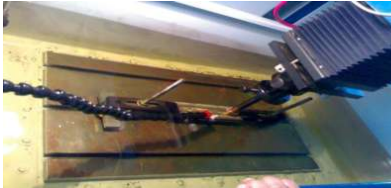
Fig IV. Setup of work piece & electrode
