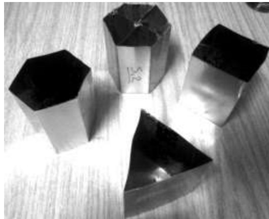
Fig.5. Fabricated samples before loading
