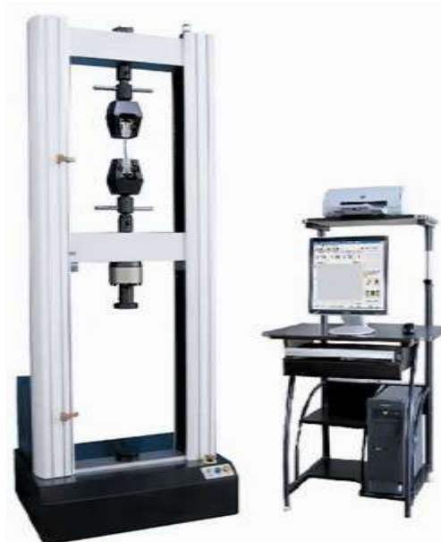
Fig.3. WDW-10 Computer Control Electromechanical Universal Testing Machine.
