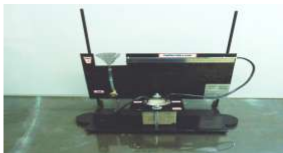
Figure 1: Initial surface absorption test apparatus
