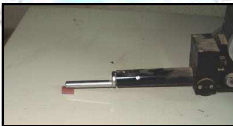
Figure (3.15): Surface roughness measurement by stylus profilometer
