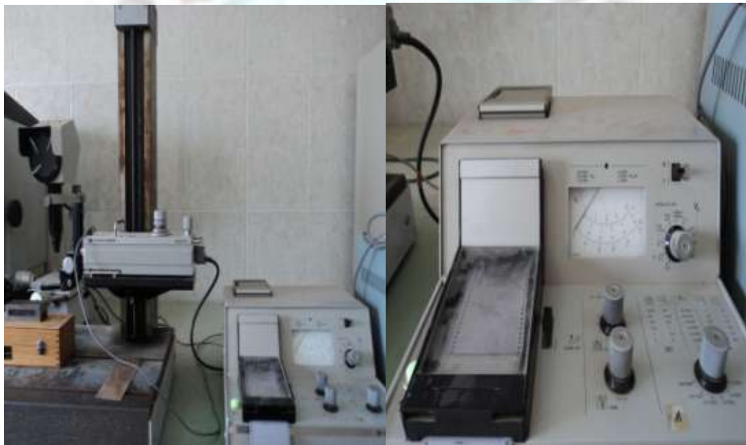
Figure (3.16): contact(stylus) profile meter surface roughness device
