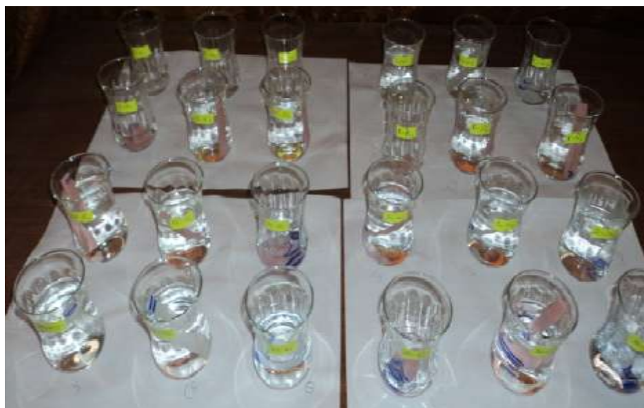
Figure(3.24) Residual monomer specimens inside glass container with distilled water
