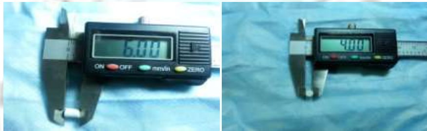
Figure (7): Specimens dimension (6mm x 4mm) according to ADA NO.96.
