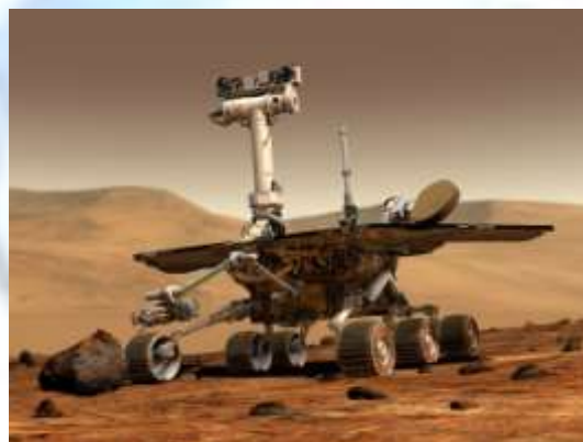
Fig.2: Artist's Concept of Rover on Mars, an example of an unmanned land-based vehicle. Notice the stereo cameras mounted on top of the Rover.
