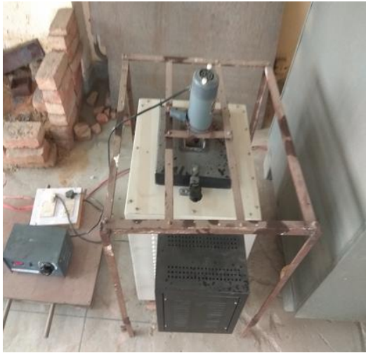
Pic. 1 Stirrer setup on muffle furnace.
