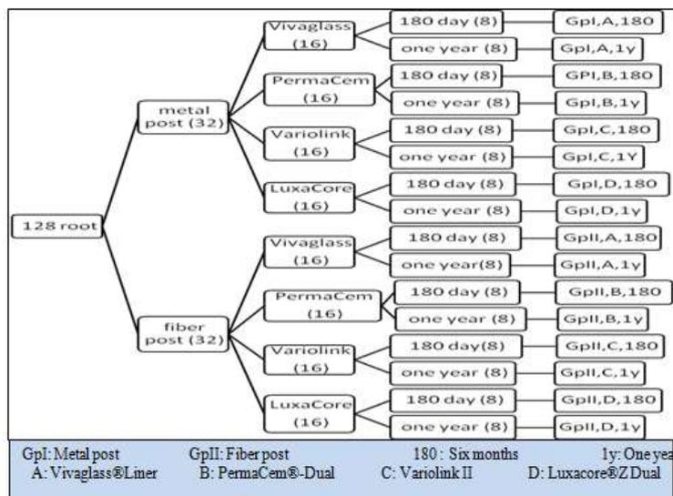
Figure (1): Diagrammatic illustration of the experimental design of groups for the study
