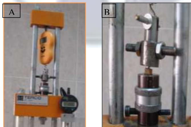
**Figure (2): (A) Tensile loading performed using a computer controlled universal testing machine (TERCO, MT, Sweden). (B) Tensile force was applied**
