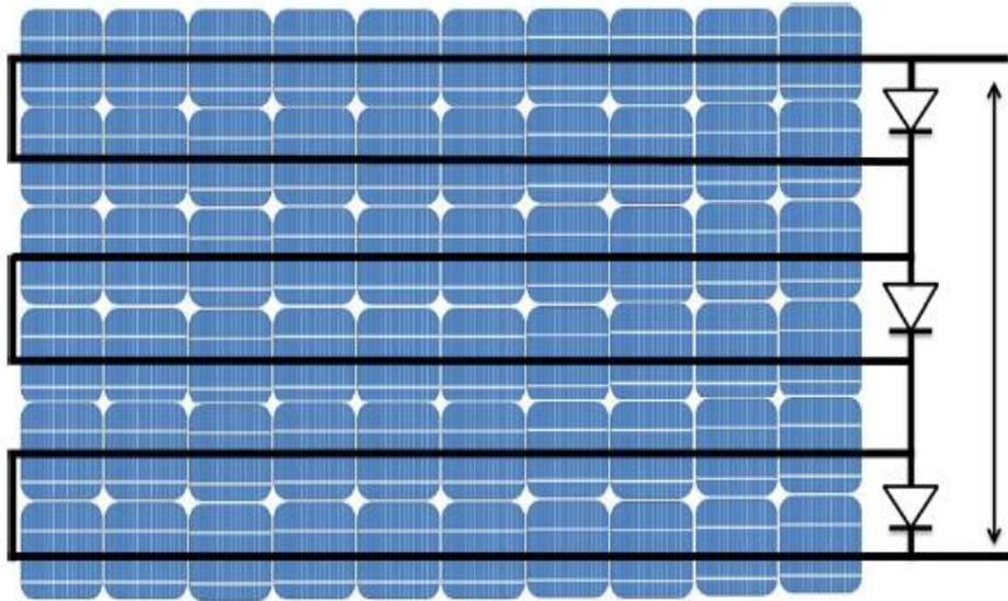
**Fig.(3) Sketch of a typical silicon wafer-based c-Si module**
