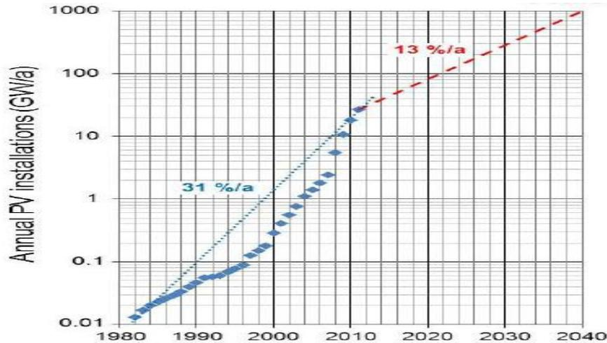
Fig.(1) Historic and expected development of the global solar PV production [3].
