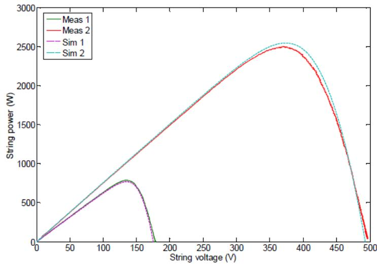
Fig.(12) Measured and Simulated PV curves of 6 modules string and 17 modules string from 26<sup>th</sup> August 2015. [26]
