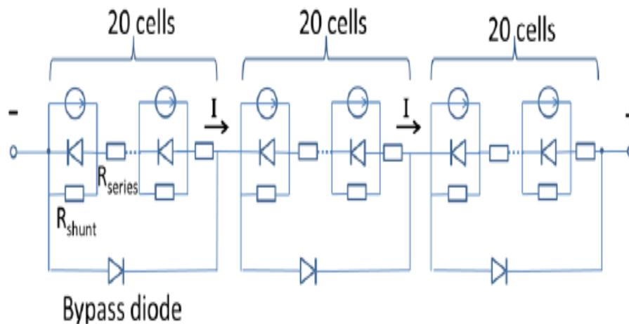
**Fig.(4) Sketch of the circuit simulation model of a silicon wafer-based PV module based on the one-diode model.**
