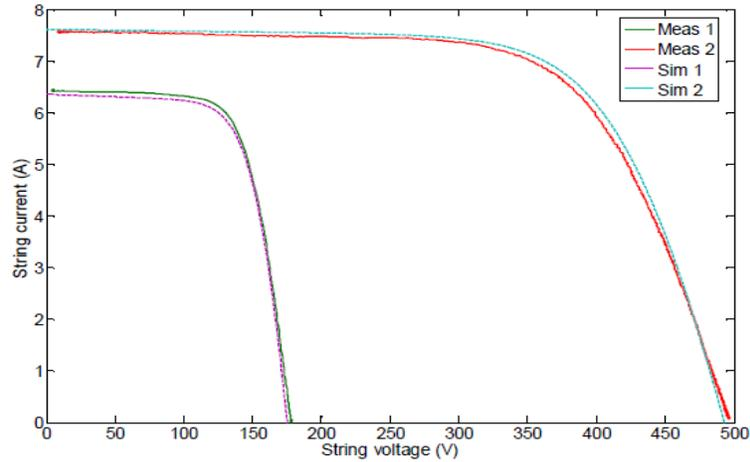
Fig.(11) Measured and simulated IV curves of the 6 modules string and the 17 modules sting from 26<sup>th</sup> August 2015.
