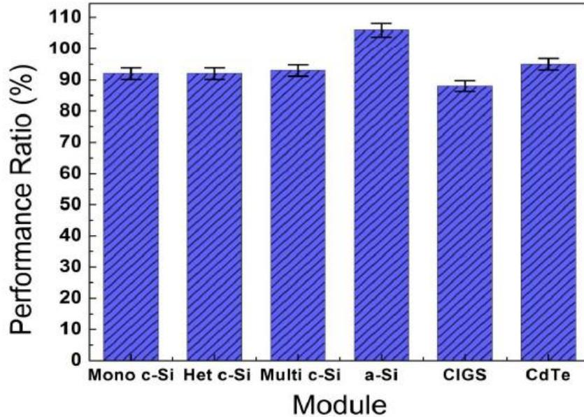
Fig.(5) DC performance ratio based on the power for individual modules.
