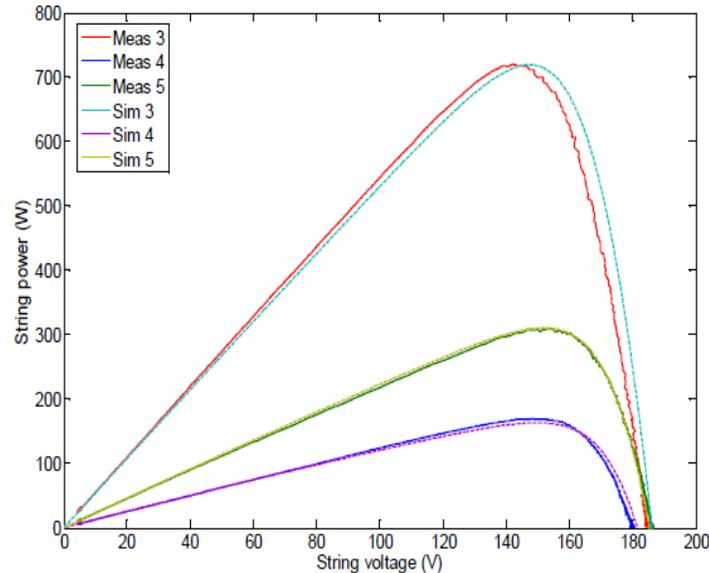
**Fig.(14) Measured and Simulated PV curves of 6 modules string from September 6<sup>th</sup> 2015.**
