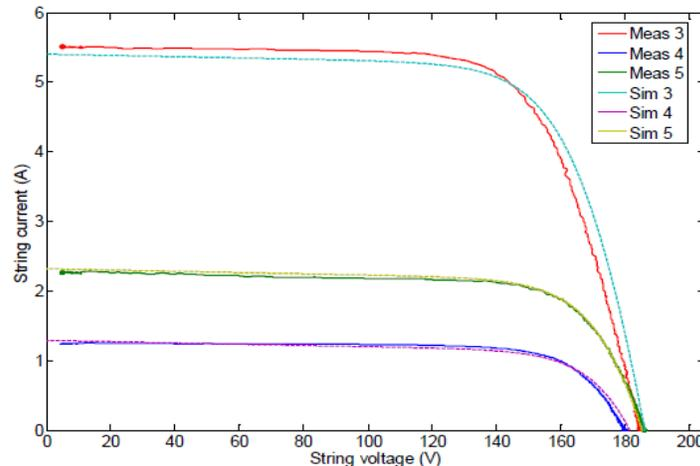
Fig.(13) Measured and Simulated IV curves of 6 modules string from September 6<sup>th</sup> 2015.
