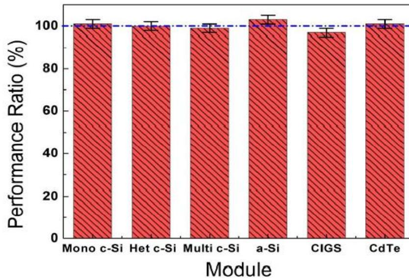
Fig.(10) Performance ratio based on newly defined Tropical Test Conditions , as proposed in this work. [25]
