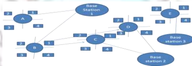
Figure 5.2 Scenario of Mobile Nodes (beacons) with base stations
