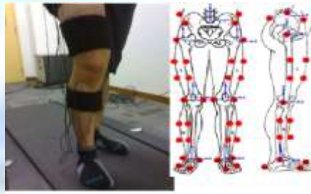
Fig.1: (a) Sensor (EMG) placement on lower limb of subject (b) Surface marker placement on lower body
