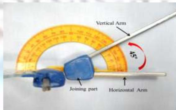
Figure (7): The joining part and the 45° vertical angulation of the beam aiming device of the longitudinal topographic occlusal projection.
