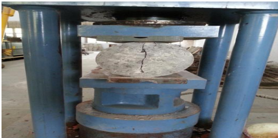
Fig 4- Split Tensile Testing
