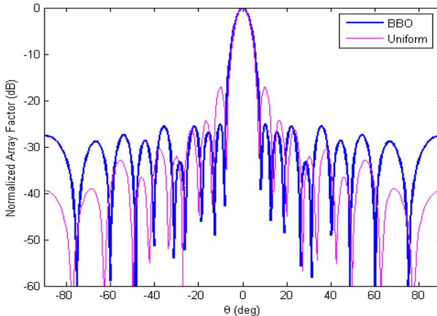
Fig. 5: Radiation pattern of CCAA with  $N_1 = 8$  and  $M = 9$
