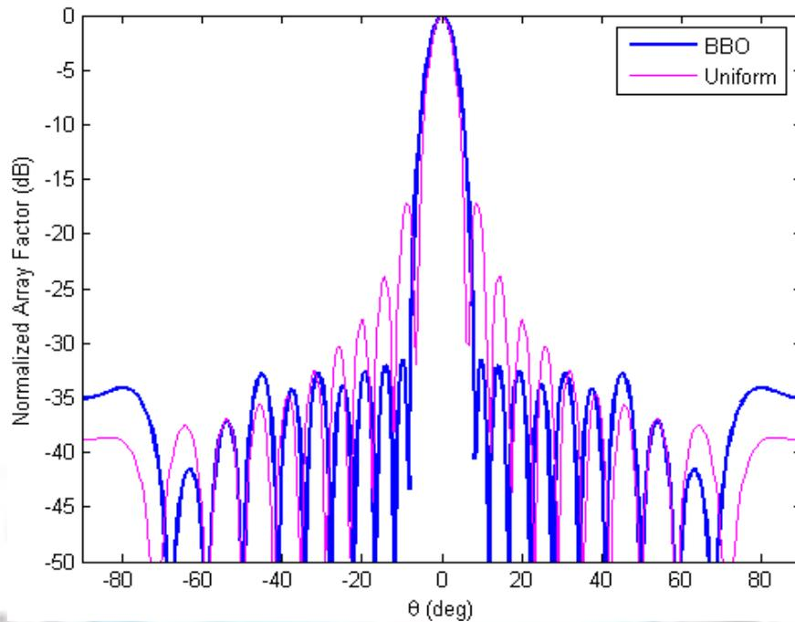
Fig. 4 Radiation pattern of CCAA with  $N_1 = 5$  and  $M = 11$
