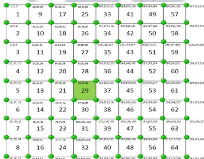
Fig. 2: Plate with 64 elements and 243 degree of freedoms.
