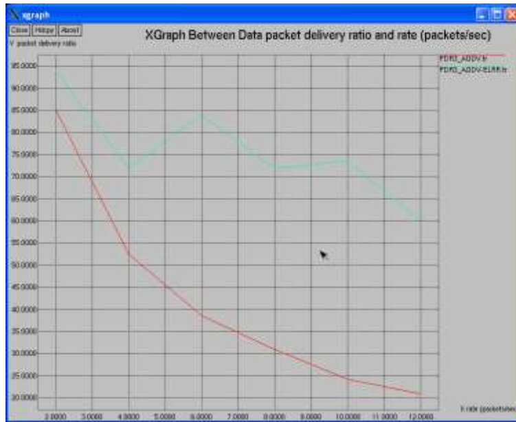
Figure2. X-graph for Packet delivery ratio v/s packet rate for 20 ms speed of nodes
