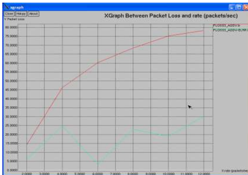
Figure 5. X-graph for packet loss v/s packet rate for 20 ms speed of nodes
