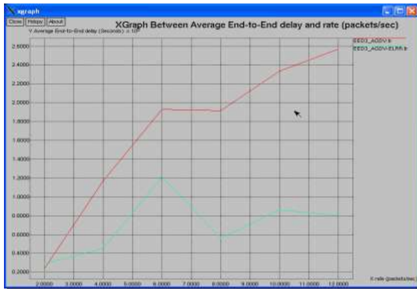
Figure4. X-graph for average end to end delay v/s packet rate for 20 ms speed of nodes
