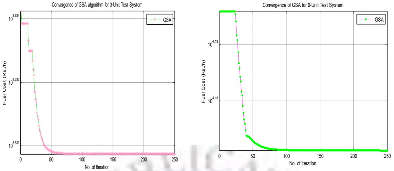
**Fig.4: Convergence of GSA algorithm for 3 and 6-Generating Unit Systems**
