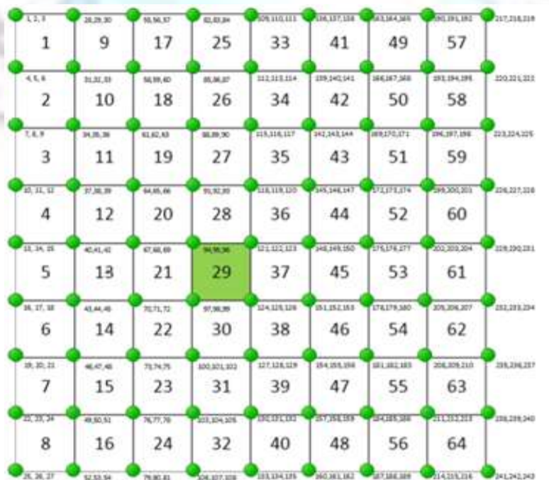
Fig. 2: Plate with 64 elements and 243 degree of freedoms.
