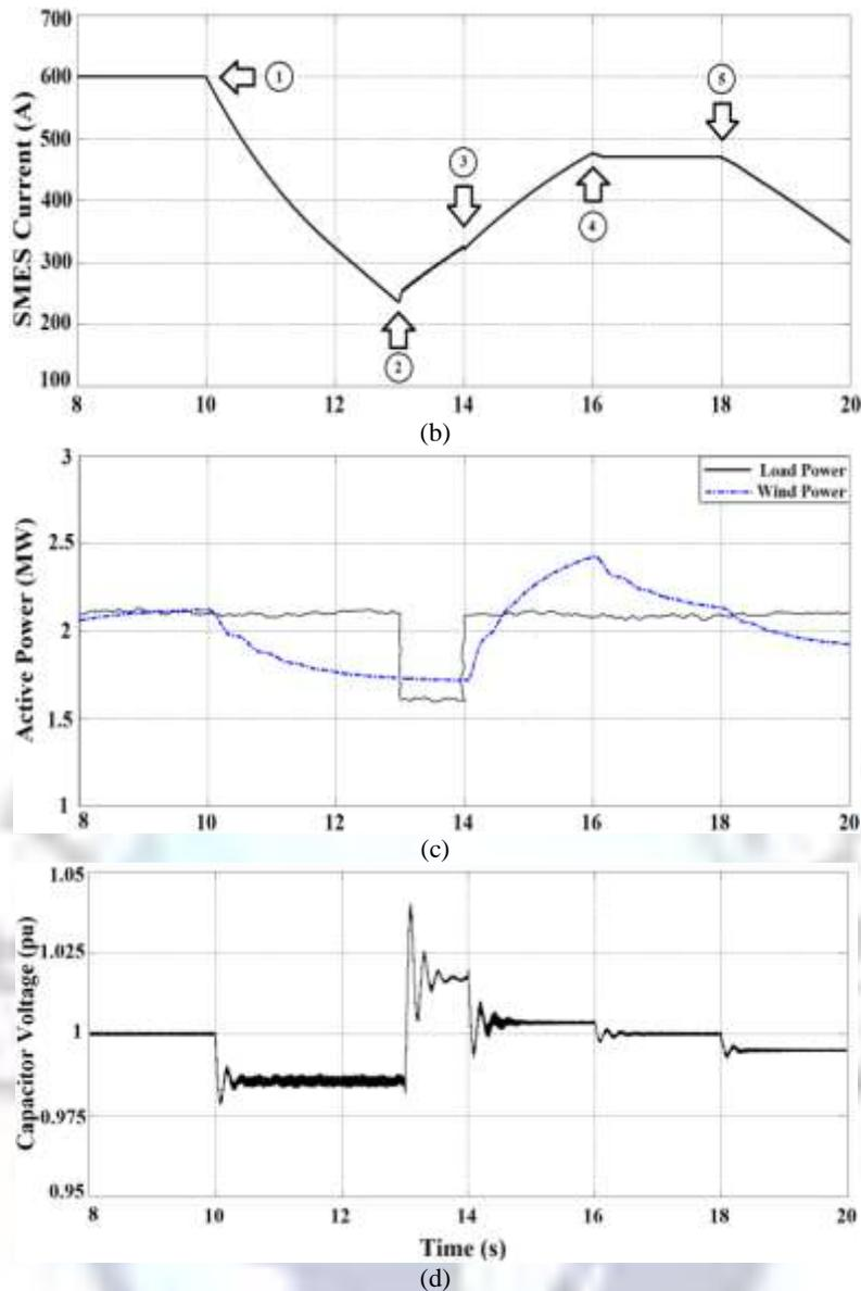
**Figure 10.** System operation during prolonged low-wind mode (Case 2). (a) Wind speed. (b) SMES coil current. (c) Power generated by the wind turbine and total load. (d) DC-link voltage.
