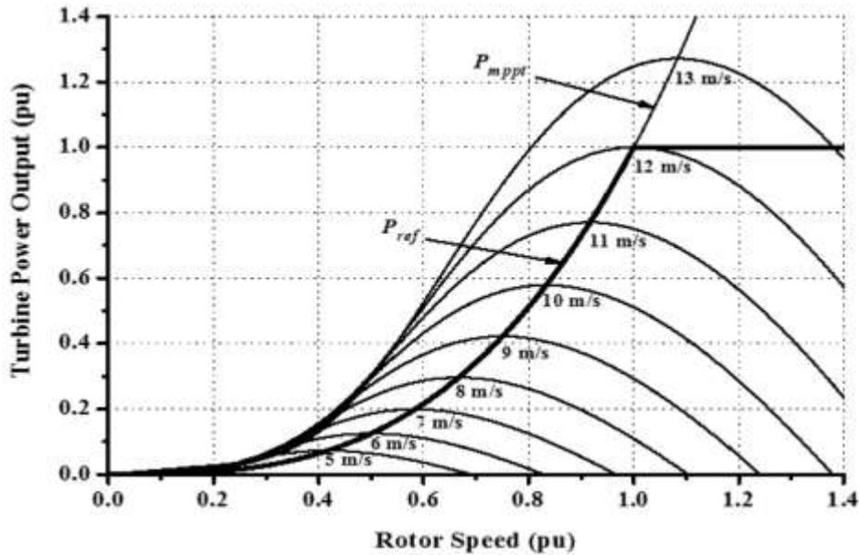
Figure 2. characteristic of Turbine power ( $\beta=0^\circ$ ) [20].
