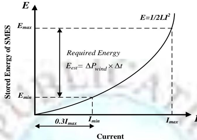
**Figure 4.** Estimated energy of the SMES according to lower and upper coil current limits (Adapted from [12]).
