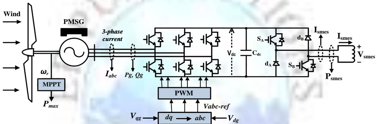
**Figure 6. Control diagram of PMSG-based variable speed wind turbine**
