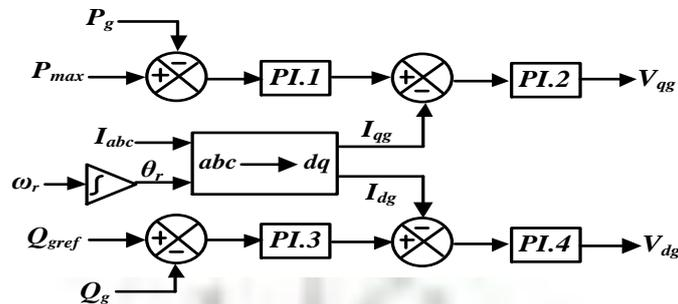
**Figure 5. Generator side controller of PMSG.**
