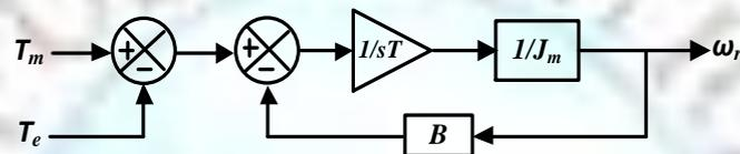
Figure 3. Modeling of wind turbine system drive-train.
