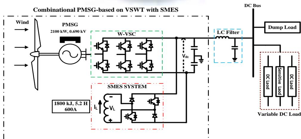
**Figure 1. Combination of PMSG- based on VSWT and SMES system in dc microgrid.**
