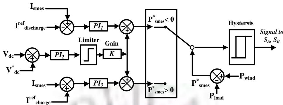
Figure 7. Control diagram of dc-dc converter with SMES coil.
