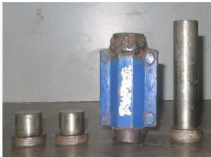
Fig. 2 Cast iron mould with detachable collars for UCS sample
