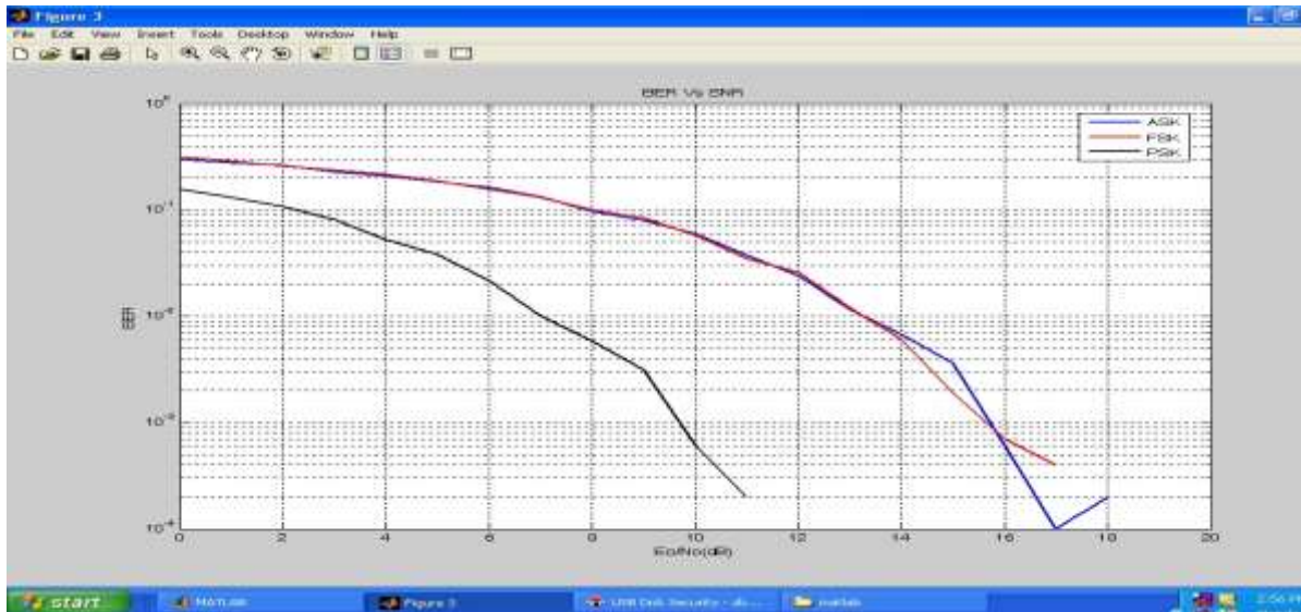
Fig 4.: BER vs. Signal to Noise ratio of different modulation techniques
