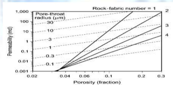
Figure (1): Variations of pore-throat size with permeability and porosity. (After Lucia, 2007) <sup>2</sup>
