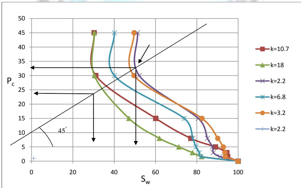
Figure (4): Capillary Pressure Relation with Water Saturation for well NR19
