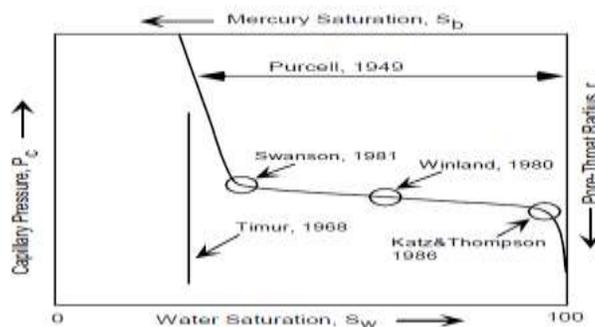
Figure(2): An idealized capillary pressure curve showing used by different aurtthors for determination of characteristic pore dimension (modified from Nelson,1949).<sup>12</sup>
