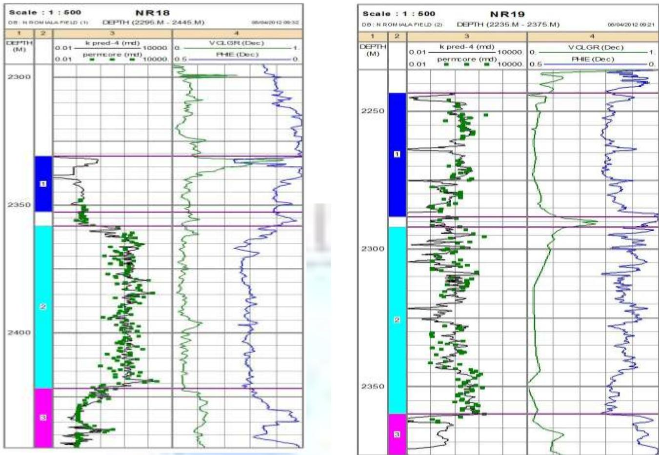
Figure(5): Predicted and measured permeability for wells: NR18 and NR19, by using Eq.(16) with coefficient in the table (4).
