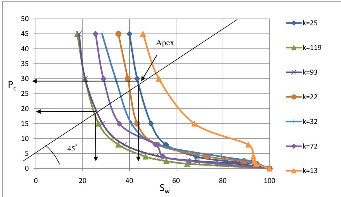
Figure (3): Capillary Pressure Relation with Water Saturation for well NR18
